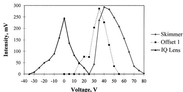
Fig. 5. Plot illustrating the effect of voltage settings on gramicidin S signal intensity. Conditions: gramicidin S ( $10 \mu\text{M}$ ) in  $\text{CH}_3\text{OH}$ –water– $\text{CH}_3\text{COOH}$  (70:30:0.1, v/v); continuous infusion ( $0.3 \mu\text{l min}^{-1}$ );  $\mu\text{ESI}$  (2100 V),  $30^\circ\text{C}$ ; MS data acquisition at 5000 Hz pulsing rate, 5000 spectra averaged,  $1 \text{ spectrum s}^{-1}$ .
