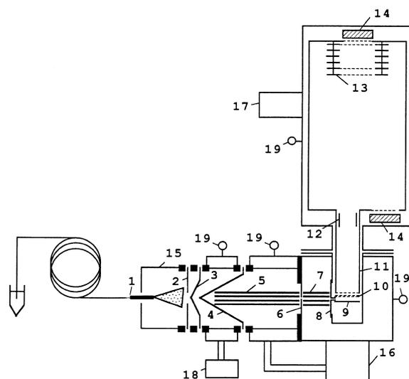
Fig. 1. Schematic diagram of the ESI-TOF-MS system. (1) Electro spray needle, (2) interface plate, (3) nozzle, (4) skimmer, (5, 7) RF-only quadrupoles, (6) interquad lens, (8) slit/lens, (9) pulser, (10) grids, (11) flight tube, (12) deflection plates, (13) reflectron, (14) electron multiplier, (15) ion source, (16, 17) turbo pumps, (18) rotary pump, (19) vacuum gauge.
