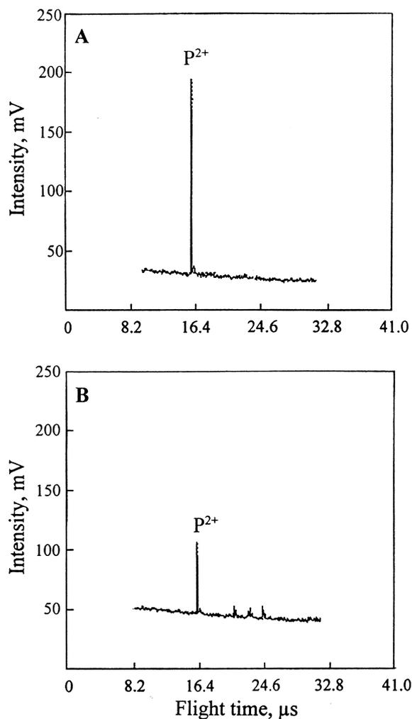
Fig. 4. TOF mass spectra illustrating the effect of pressure in the second vacuum stage on transmission of paraquat ion. Conditions: Paraquat (50  $\mu$ M) in  $\text{CH}_3\text{OH}$ -water- $\text{CH}_3\text{COOH}$  (70:30:0.1, v/v); continuous infusion ( $0.3 \mu\text{l min}^{-1}$ );  $\mu$ ESI (2150 V), 40°C; MS data acquisition at 5000 Hz pulsing rate, 5000 spectra averaged, 1 spectrum  $\text{s}^{-1}$ ; (A)  $3 \cdot 10^{-2}$  Torr; (B)  $1.2 \cdot 10^{-1}$  Torr.
